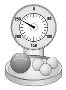
The dial on the weighing machine shows weight in grams (g).
